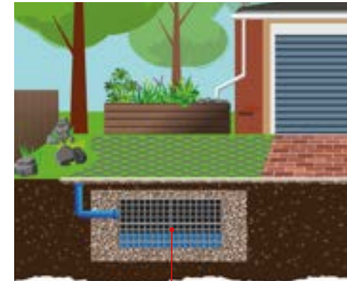
Below ground runoff storage and attenuation crates
